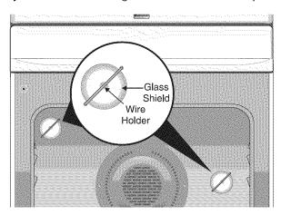
**ACAUTION** Be sure the range is unplugged and all parts are COOL before replacing oven light. Wear a leather-faced glove for protection against possible broken glass.
